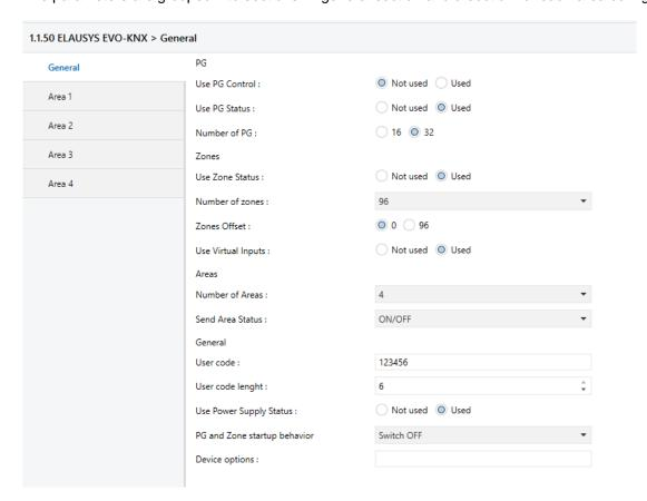
In the general section, enter a valid user code from the Paradox system to enable area control.
