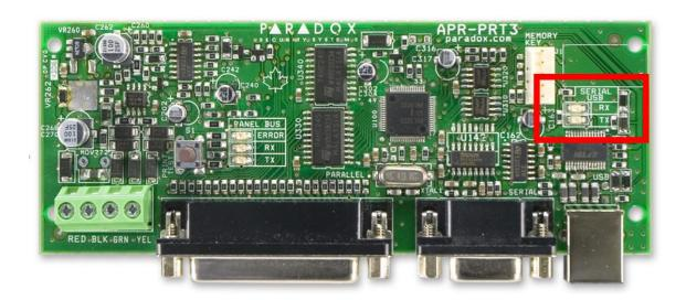
These LEDs can be used to see if the PRT3 module correctly sends status to the EVO-KNX. When zone reporting is configured, opening or closing a zone should make the TX LED blink once. If this is not the case, the PRT3 configuration is not correct. Verify that all required settings are done according to chapter 2.3.
